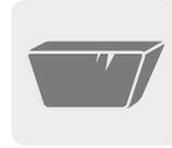
If, in the course of time, the stone resin gets chipped – for example by being hit forcefully by a hard object – we offer you a **stone resin repair set** free of charge. You can easily repair small patches using this repair set. It includes a stone resin mixture and fine sandpaper, with which you can create an invisible transition at the damaged site.
