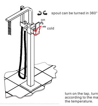
turn on the tap, turn the handle according to the marks to adjust the temperature.
