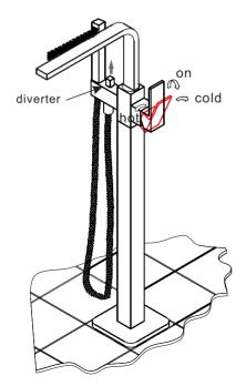
switch between tap and hand shower by push and pull the diverter.
